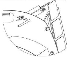
A: Feed label liner over strip plate separating the liner from the label
