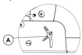
A: To apply the proper amount of tension for proper label feeding and detection; loosen brush wing screw and press down to increase tension, then tighten screw.
