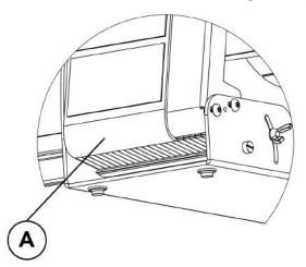
A: Feed label liner between brush and strip plate
