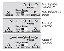
Note: Terminals are #6 screws. DC contacts are polarity sensitive.
