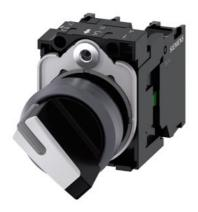
Selector switch, illuminable, 22 mm, round, plastic with metal front ring, white, selector switch, short, 2 switch positions O-I, latching, actuating angle 90°, 10:30h/13:30h, with holder, 1 NO, 1 NC, screw terminal
