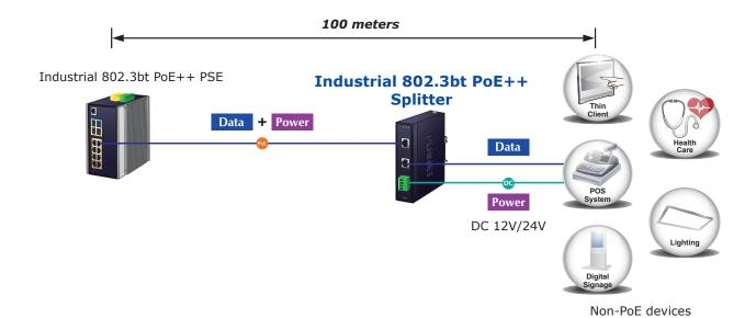
The POE-173S frees the network device deployment from restrictions of power outlet locations, thus eliminating the costs for additional AC wiring and reducing the installation time.
