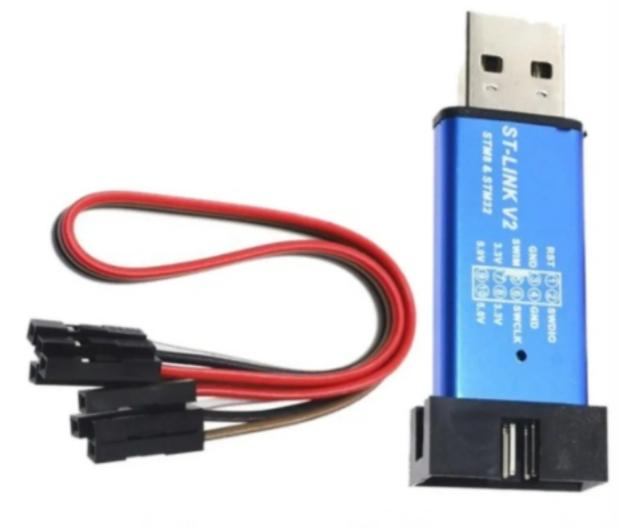
USB In-Circuit Programmer and Debugger compatible with ST-LINK V2 for the STM8 and STM32 microcontroller families.
