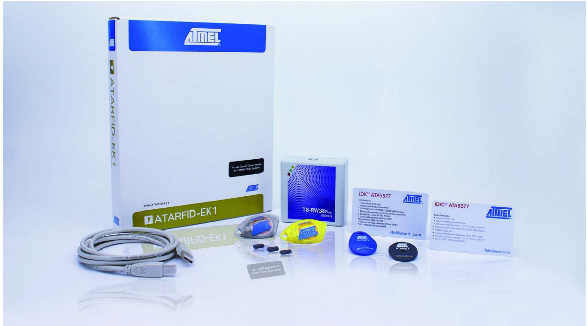
Figure 2-1. Content of the Atmel ATARFID-EK1: 125kHz Kit
