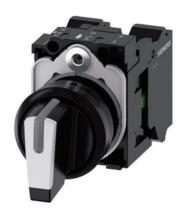
Selector switch, illuminable, 22 mm, round, plastic, white, selector switch, short, 3 switch positions I-O-II, latching, 10:30h/12h/13:30h, with holder, 1 NO, 1 NO, spring-type terminal, Z=20-unit packaging
