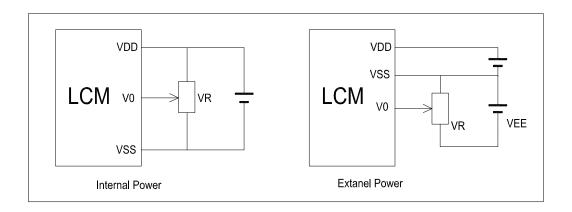
V<sub>DD~</sub>V<sub>0</sub>: LCD Driving voltage
