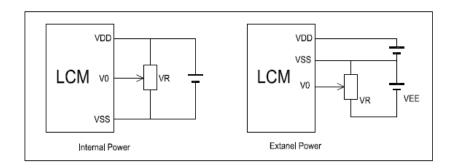
$V_{DD\sim}V_0$ : LCD Driving voltage
