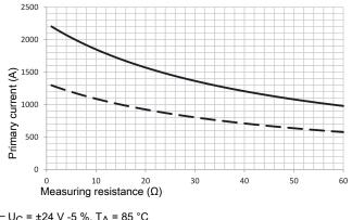
$\begin{array}{l} ---- U_C = \pm 24 \; V \; -5 \; \%, \; T_A = 85 \; ^\circ C \\ ---- U_C = \pm 15 \; V \; -5 \; \%, \; T_A = 85 \; ^\circ C \\ \mbox{Primary currents higher than } I_{PM} \; \mbox{only for peak!} \end{array}$
