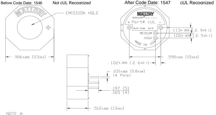
NOTE A: TERMINALS - .031″ DIA. NICKEL/TIN COATED BRASS. NOTE R:
