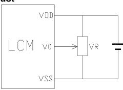
VDD~V0: LCD Driving voltage
