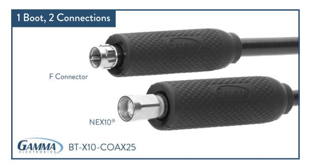
Gamma's NEX10 & F Connector Weatherproof Boot is an IP68 rated boot that works on both NEX10 and F Connections. It typically comes pre-installed on the cable allowing it to slide up and over the connection creating a watertight seal. As part of the IP68 testing process the boot has been placed in water tanks more than 1 meter in depth for over 30 min without showing any signs of water ingress.
