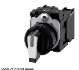
Selector switch, illuminable, 22 mm, round, plastic, white, selector switch, short, 3 switch positions I>O<II, momentary contact type, 10:30h/12h/13:30h, with holder, 1 NO, 1 NO, screw terminal, Z=20-unit packaging
