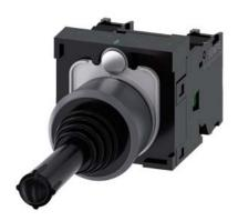
Coordinate switch, 22 mm, round, plastic with metal front ring, black, 2 switch positions, vertical latching, without mechanical interlocking, in O position, with holder, 1 NO, 1 NO, screw terminal, with laser labeling, lower case
