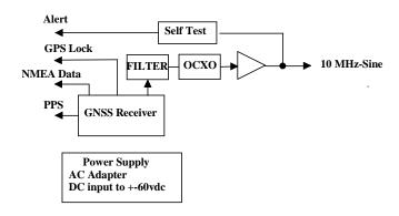
The signal source is a GNSS-driven, mixed-signal, phase-lock-loop generating a 10 MHz sine output from an intrinsically low jitter OCXO-controlled crystal oscillator. The output is a 0.4 Vrms sine.
