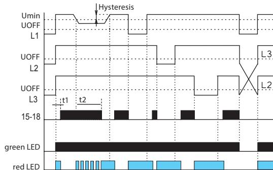
**Voltage Monitoring** Three-phase monitor confirms correct sequence and detects failure of any one phase. Phase failure results in a flashing red LED and opening of output relay.
