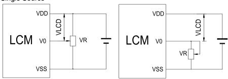
V<sub>DD∼</sub>V₀: LCD Driving voltage
