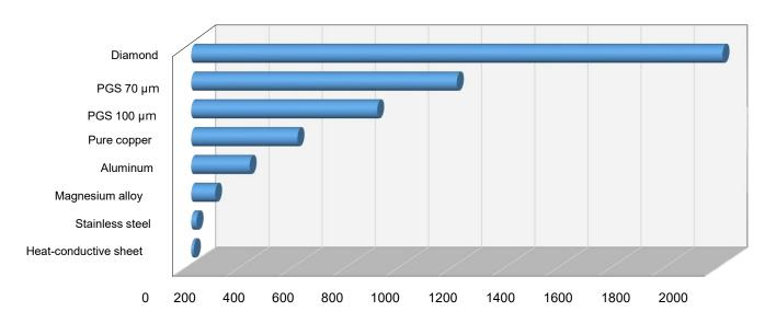
Coefficient of thermal conductivity W / (m·K)
