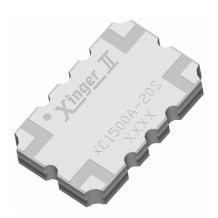
The XC1500A-20S is a low profile, high performance 20dB directional coupler in a new easy to use, manufacturing friendly surface mount package. It is designed for AMPS band applications. The XC1500A-20S is designed particularly for power and frequency detection, as well as for VSWR monitoring, where tightly controlled coupling and low insertion loss is required. It can be used in high power applications up to 160 Watts.
