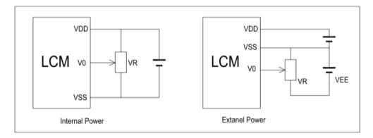
VDD-V0: LCD Driving Voltage VR: 10k-20k
