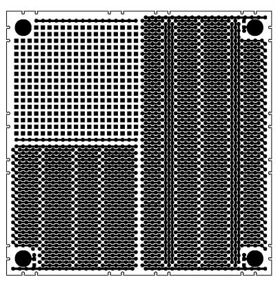
Through Hole 0.1" Spacing Including Schmartboard's Signature 0.05" Offset Grid, 4" X 4"
