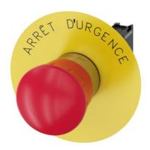
EMERGENCY STOP mushroom pushbutton, 22 mm, round, metal, shiny, red, 40 mm, positive latching, acc. to EN ISO 13850, rotate-to-unlatch, with yellow backing plate, inscription: Arrêt d'urgence, with holder, 1 NC, screw terminal, Z=20-unit packaging
