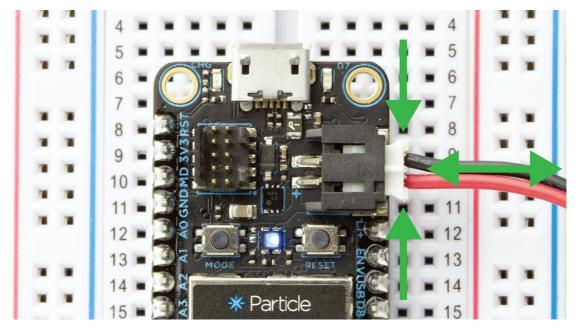
The micro B USB connector on the Boron is soldered on the PCB with large surface pads as well as couple of through hole anchor points. Despite this reinforcement, it is very easy to rip out the connector if too much stress is put on in the vertical direction.
