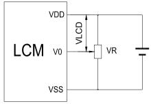
V<sub>DD~</sub>V₀: LCD Driving voltage
