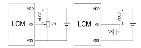
$V_{DD^{\sim}}V_{0}\text{: }LCD\text{ }Driving\text{ }voltage$
