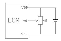
VDD~V0: LCD Driving voltage
