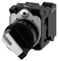
Selector switch, illuminable, 22 mm, round, plastic, white, selector switch, short, 2 switch positions O-I, latching, 10:30h/13:30h, with holder, 1 NO, spring-type terminal, with laser labeling, upper case
