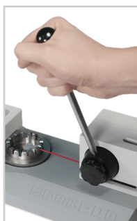
Ergonomic lever easily applies force and releases the sample.
