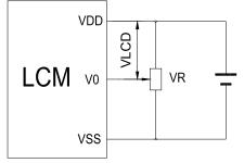
$V_{DD-}V_0$ : LCD Driving voltage VR: 10k~20k
