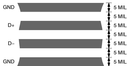
Figure 28. Arrangement of Signal Tracks
