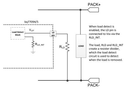
Figure 11. Load Detection Circuit For Current Faults Recovery
