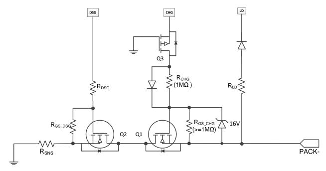
Figure 23. Optional Components Combining Figure 21 and Figure 22 Protections
