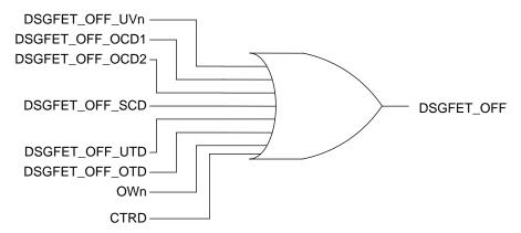
Figure 14. Faults That Can Qualify DSGFET OFF
