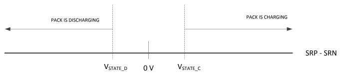
Figure 13. State Comparator Thresholds
