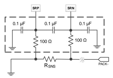
Figure 26. Optional Filters Improve Current Measurement
