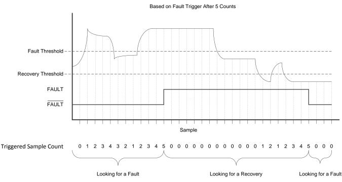
Figure 12. Fault Trigger Filtering
