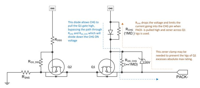
Figure 22. Protect CHG FET from High Voltage on PACK-
