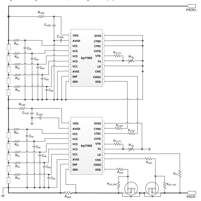
Figure 17. 10S Pack Using Two bq77905 Devices
