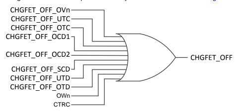
Figure 15. Faults That Can Qualify CHGFET OFF
