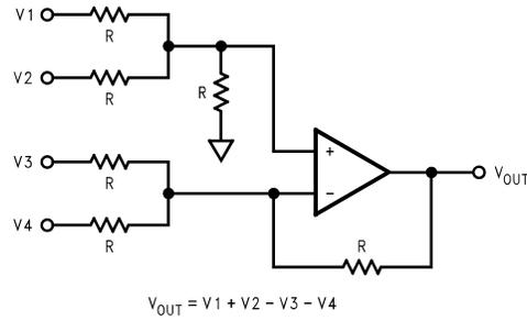
**Figure 40. Adder/Subtractor Circuit**
