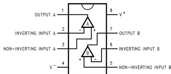
**Figure 1. 8-Pin PDIP/SOIC/VSSOP Package**
