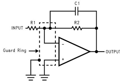
**Figure 33. Inverting Amplifier**
