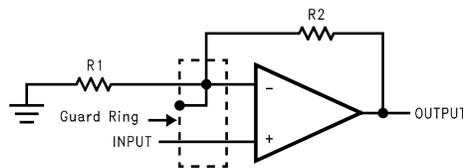
**Figure 34. Non-Inverting Amplifier**
