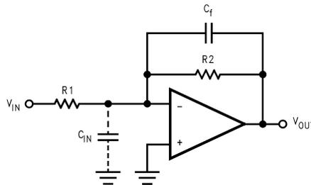
**Figure 30. Cancelling the Effect of Input Capacitance**
