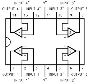
**Figure 2. 14-Pin PDIP/SOIC Package**
