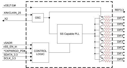
Note: Resistors default to internal on 41/51 devices. P1 devices have programmable default impedances on an output-by-output basis.
