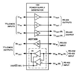
The RS-232 channels are suitable for communications rates up to 100 kHz and the RS-422 channels are suitable for high speed communications up to 5 MHz. The RS-422 transmitter complementary outputs are closely matched and feature low timing skew between the complementary outputs. This is often an essential requirement to meet tight system timing specifications.
