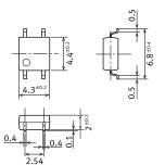
Terminal thickness: t = 0.15 General tolerance: ±0.1
