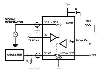
FIGURE 5. CROSSTALK TEST CIRCUIT
