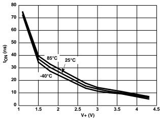
FIGURE 12. TURN - ON TIME vs SUPPLY VOLTAGE
