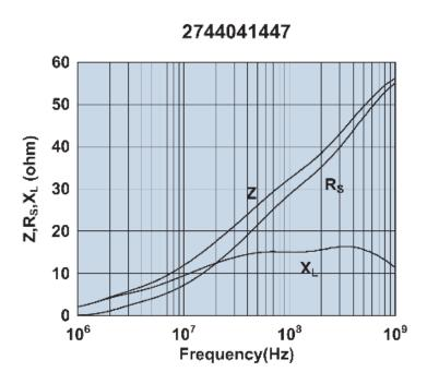
Impedance, reactance, and resistance vs. frequency.
