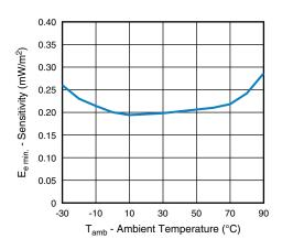
Fig. 9 - Sensitivity vs. Ambient Temperature
