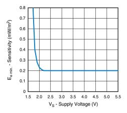
Fig. 13 - Sensitivity vs. Supply Voltage
