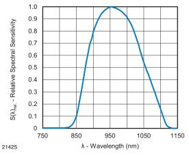
Fig. 10 - Relative Spectral Sensitivity vs. Wavelength
