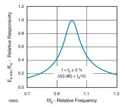
Fig. 5 - Frequency Dependence of Responsivity
