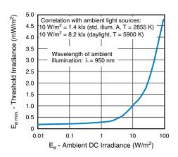
Fig. 6 - Sensitivity in Bright Ambient
