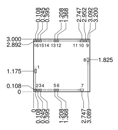
Unit: millimeters Thickness: 0.10
