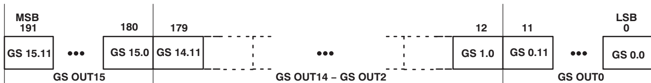
Figure 18. Grayscale Data Packet Format
