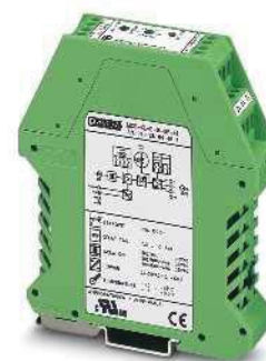
For sinusoidal alternating currents, 0 ... 16 A AC
