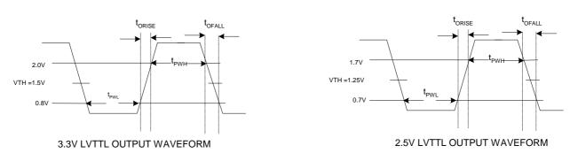
Figure 4. Test Waveforms
