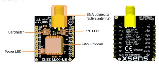
Figure 10: Top view (left) and the bottom view (right) of the GNSS daughter card
