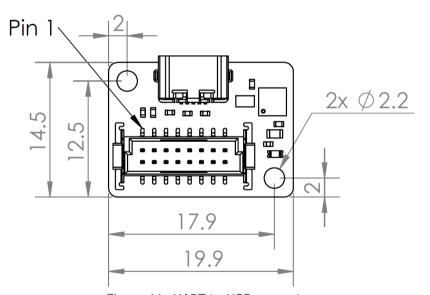
Figure 11: UART to USB converter.
