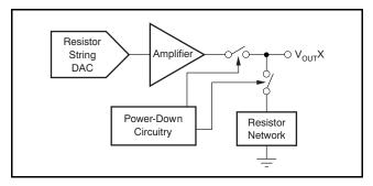
Figure 96. Output Stage During Power-Down
