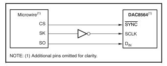
Figure 102. DAC8564 to Microwire Interface
