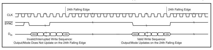
Figure 95. SYNC Interrupt Facility
