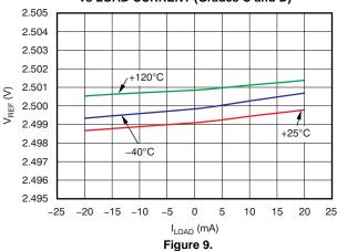
INTERNAL REFERENCE VOLTAGE vs LOAD CURRENT (Grades A and B)
