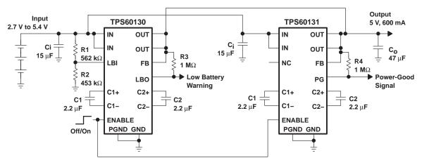
Figure 25. Paralleling of Two TPS6013x Charge Pumps
