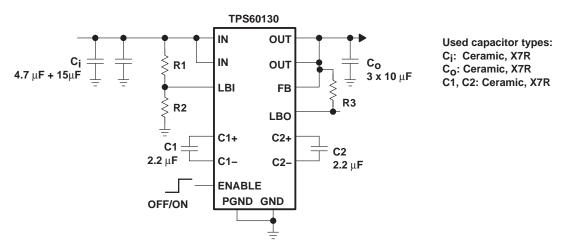
Figure 5. Circuit Used For Typical Characteristics Measurements
