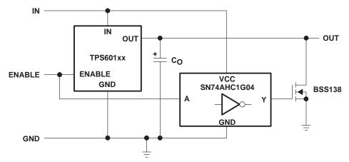
Figure 27. Block Diagram of the Regulated Discharge of the Output Capacitor
