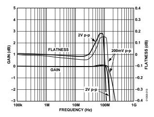
Figure 13. AD8109 Frequency Response
