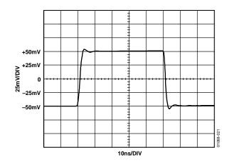
Figure 16. AD8109 Step Response, 100 mV Step
