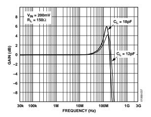
Figure 32. AD8108 Frequency Response vs. Capacitive Load
