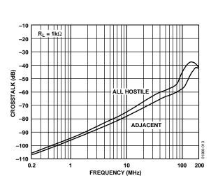
Figure 8. AD8108 Crosstalk vs. Frequency
