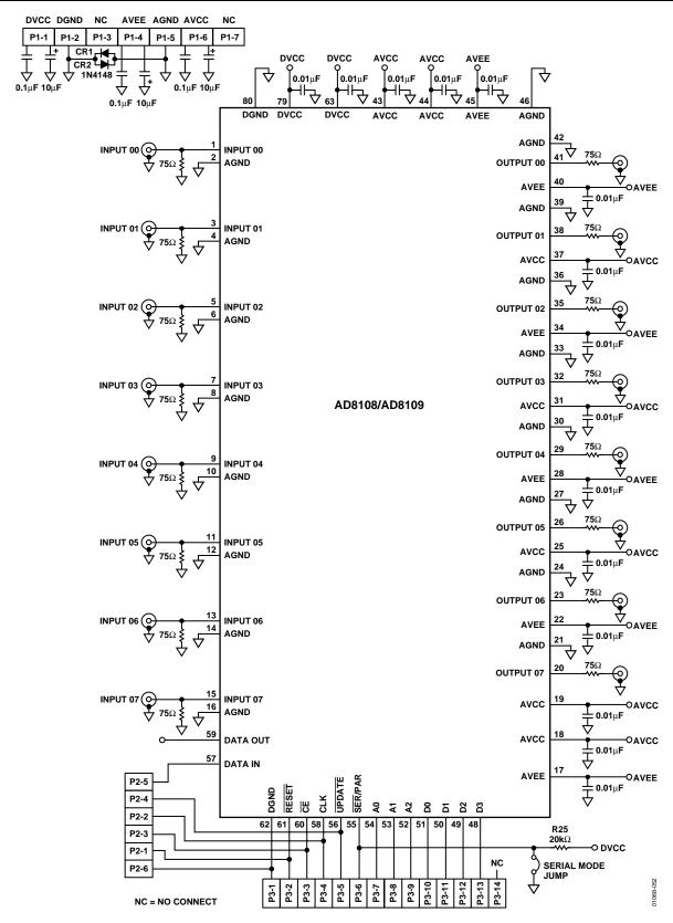
Figure 60. Evaluation Board Schematic
