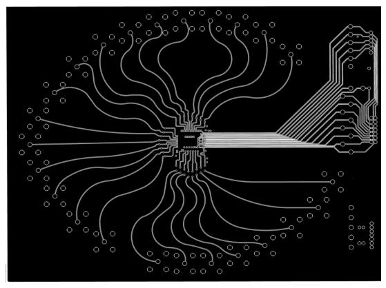
Figure 55. Board Layout (Signal Layer)
