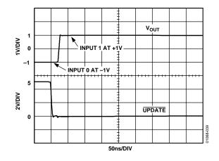
Figure 34. AD8108 Switching Time
