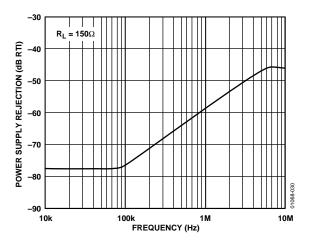
Figure 25. AD8109 PSRR vs. Frequency
