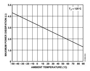
Figure 5. Maximum Power Dissipation vs. Temperature
