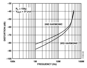
Figure 15. AD8109 Distortion vs. Frequency
