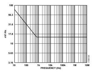
Figure 20. AD8108 Voltage Noise vs. Frequency
