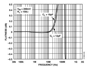
Figure 33. AD8108 Flatness vs. Capacitive Load
