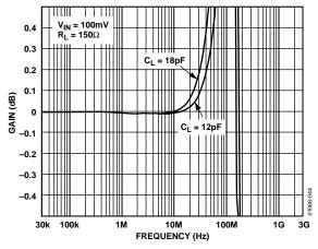
Figure 39. AD8109 Flatness vs. Capacitive Load
