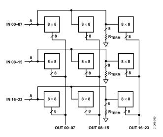
Figure 50. 24 × 24 Crosspoint Array Using Nine AD8108s or AD8109s
