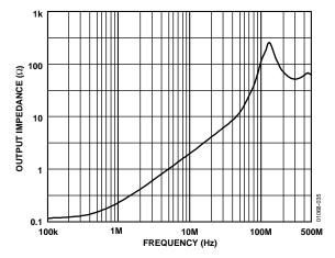
Figure 30. AD8109 Output Impedance, Enabled
