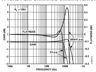
Figure 7. AD8108 Frequency Response
