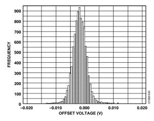
Figure 35. AD8108 Offset Voltage Distribution
