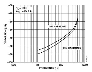
Figure 9. AD8108 Distortion vs. Frequency
