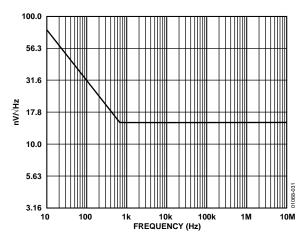
Figure 26. AD8109 Voltage Noise vs. Frequency
