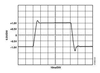
Figure 17. AD8109 Step Response, 2 V Step
