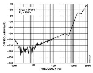
Figure 29. AD8109 Off Isolation, Input-Output
