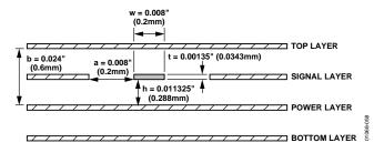
Figure 52. Cross Section of Input and Output Traces
