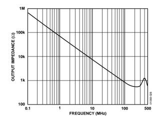
Figure 21. AD8108 Output Impedance, Disabled
