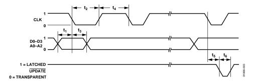
Figure 3. Timing Diagram, Parallel Mode
