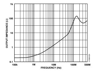
Figure 24. AD8108 Output Impedance, Enabled
