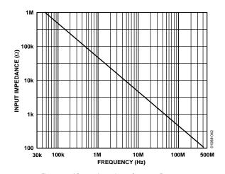
Figure 37. AD8109 Input Impedance vs. Frequency
