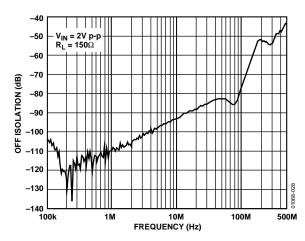
Figure 23. AD8108 Off Isolation, Input-Output
