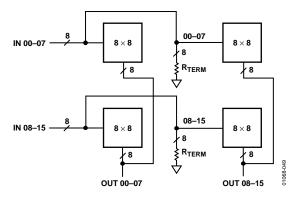
Figure 49. 16 × 16 Crosspoint Array Using Four AD8108s or AD8109s
