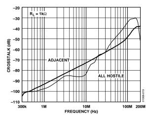
Figure 14. AD8109 Crosstalk vs. Frequency
