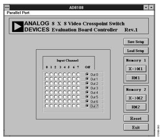
Figure 59. Evaluation Board Control Panel
