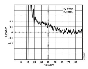
Figure 12. AD8108 Settling Time
