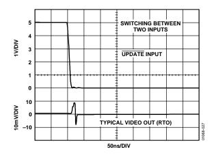
Figure 22. AD8108 Switching Transient (Glitch)
