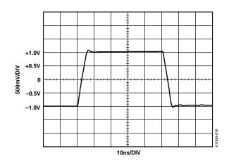
Figure 11. AD8108 Step Response, 2 V Step
