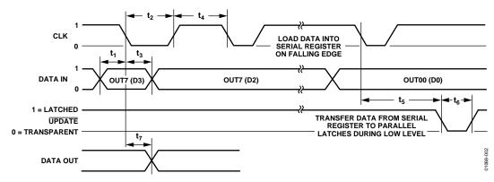
Figure 2. Timing Diagram, Serial Mode
