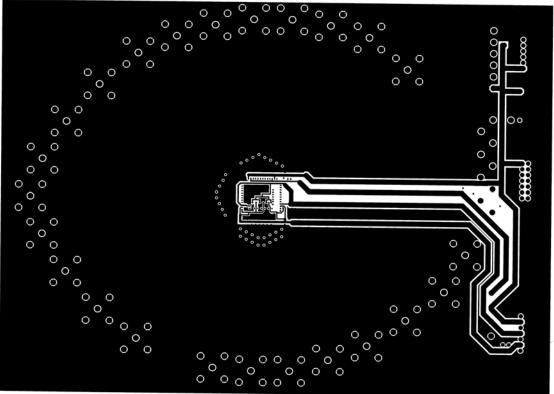
Figure 56. Board Layout (Power Plane)
