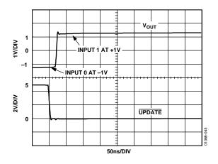
Figure 40. AD8109 Switching Time
