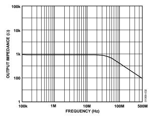
Figure 27. AD8109 Output Impedance, Disabled
