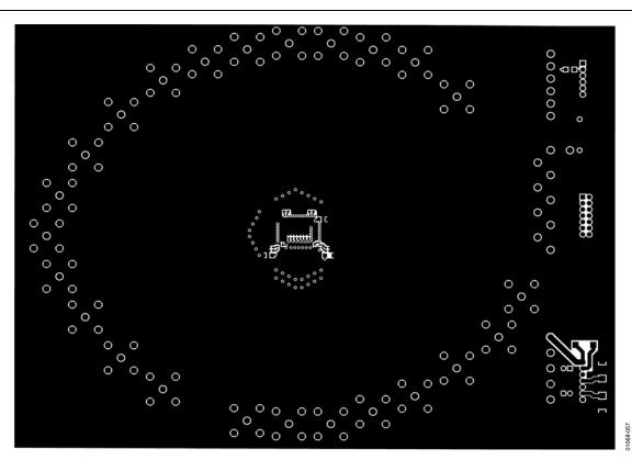
Figure 57. Board Layout (Bottom Layer)
