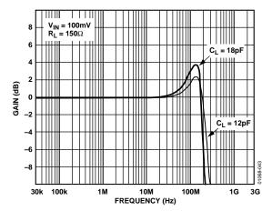
Figure 38. AD8109 Frequency Response vs. Capacitive Load
