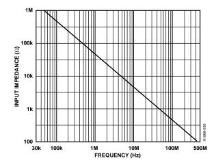
Figure 31. AD8108 Input Impedance vs. Frequency
