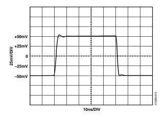
Figure 10. AD8108 Step Response, 100 mV Step
