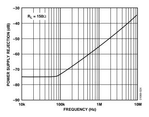
Figure 19. AD8108 PSRR vs. Frequency
