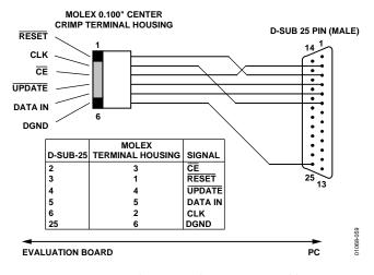
Figure 58. Evaluation Board-PC Connection Cable
