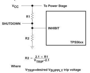
Figure 4. Input Undervoltage Lockout Circuit Using INHIBIT
