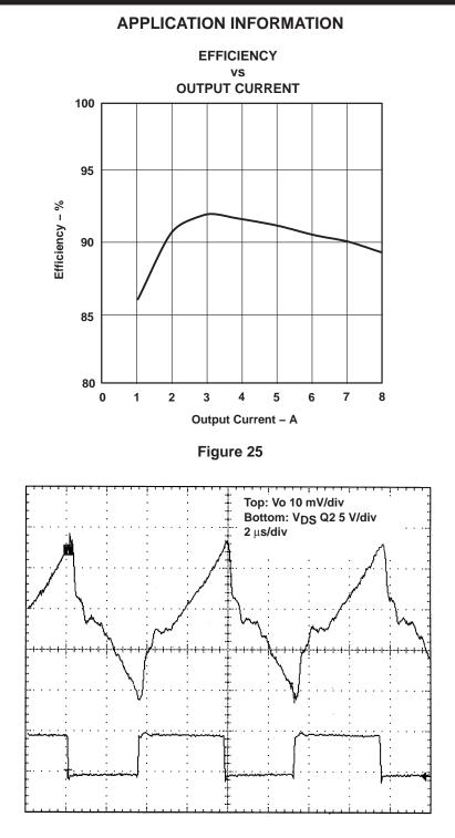
Figure 26. Output Voltage Ripple at 8 A
