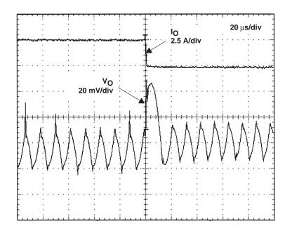
Figure 28. Falling Load Transient Response
