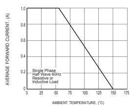
FIG.2 TYPICAL FORWARD CURRENT DERATING CURVE
