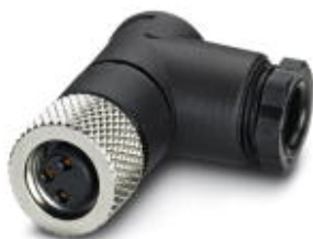
Connector, Universal, 3-position, Socket angled M8, Coding: A, Solder connection, knurl material: Nickel-plated brass, external cable diameter 3.5 mm ... 5 mm
